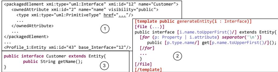
Fig. 9. Template-based code generation
